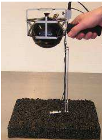
Fig. 1. Portable PU in situ measurement setup
