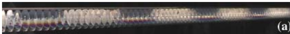
Vibrating “bamboo” foam in a tube: a standing acoustic wave is present in the tube; a swelling of the soap films is observed at the antinodes of the wave: the thicker soap films appear white on the image.
