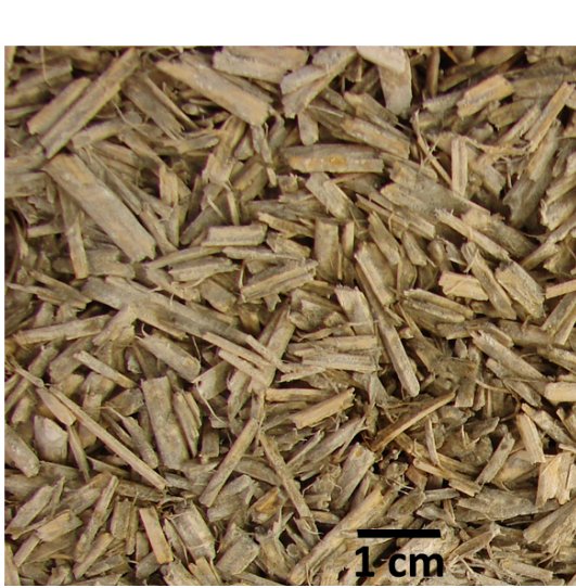
Figure 1: Hemp concrete ( left ) and modelling of hemp shiv having a density \rho = 120\text{kg/m}^3 ( right )
