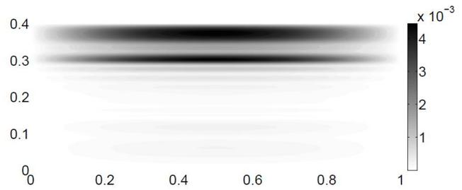
Figure 2: shear stress field at 600Hz
