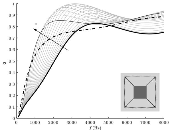
FIG. 2. Effect of the size of a square inclusion of a highly resistive porous material on the absorption coefficient. The size range from 1 to 18 mm (—) by 1 mm step. The reference homogeneous metal foam absorption is denoted by (—) and the highly resistive porous material by (---).
