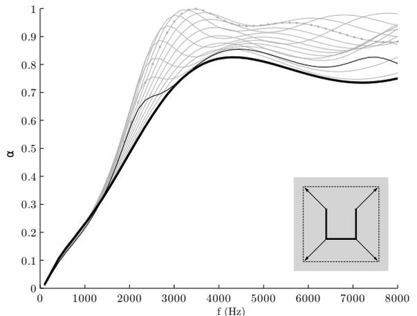
FIG. 3. Effect of the size of a rigid  $\sqcup$  inclusion on the absorption coefficient. The size range from 4 to 18 mm (—) by  $\approx 1$  mm step. The reference homogeneous metal foam absorption is denoted by (—).
